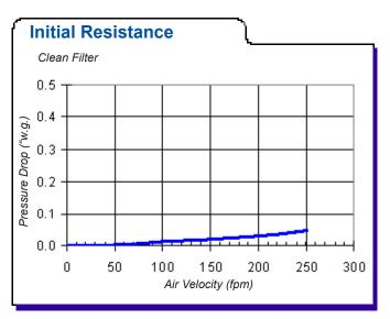
\*20" X 20" filter tested per ASHRAE 52.2, Test Aerosol KCI, Neutralized
