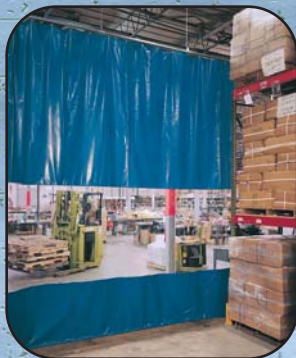
Warehouse Partition Blue vinyl laminate with clear transparent window
