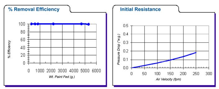
\*20" X 20" filter tested per ASHRAE 52.2, Test Aerosol KCI, Neutralized
