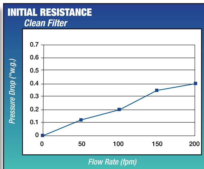
\*Filter tested per ASHRAE 52.2, Test Aerosol KCl, Neutralized. This test data is based upon clean filter performance. All filters increase in efficiency with dust loading.
